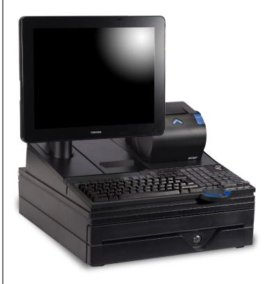
The example to the left shows the  $TCx^{TM}$  cash drawer with the black integration tray. This tray holds the TCx Display with its mount and filler, the center "credit card" filler, and the single station TCx Printer in its adapter tray.
