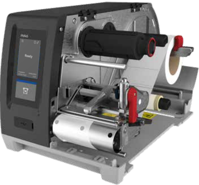
Batch Plate with Internal Rewinder The Batch Plate with Internal Rewinder is used to pre-print labels and rewind them inside the PM45. Depending on the label size up to 1/3 of a full roll can be stored inside the PM45. For full roll to roll batch printing use the Full Batch Rewinder. PM45Axxxxxx3xxxx PM45 with Internal Rewind + LTS
