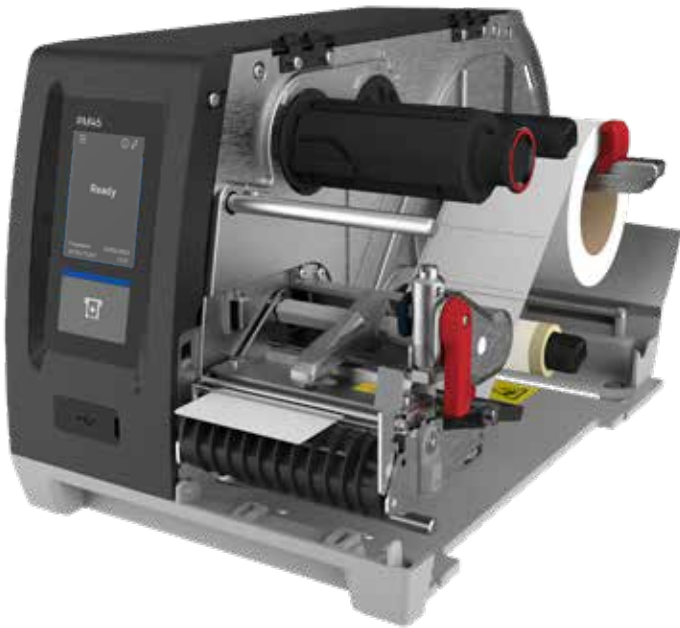
Peel & Present (Enhanced Self-Strip with Peel Off Kit) Self-Strip prints and presents only one label at a time already peeled from the backing strip/ liner, the next label will only be printed once the original label is removed from the media path. PM45Axxxxxx3xxxx PM45 with Internal Rewind + LTS 50180196-001 Label Dispenser kit
