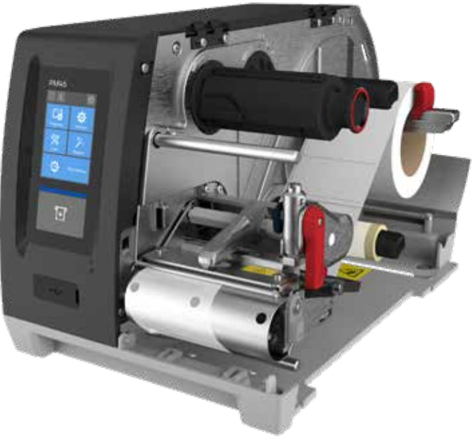
Batch Plate with Internal Rewinder The Batch Plate with Internal Rewinder is used to pre-print labels and rewind them inside the PM45. Depending on the label size up to 1/3 of a full roll can be stored inside the PM45. For full roll to roll batch printing use the Full Batch Rewinder. PM45Axxxxx3xxxx PM45 with Internal Rewind + LTS
