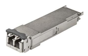
The 40GBASE-LR4-ST is a Palo Alto Networks 40GBASE-LR4 compatible fiber transceiver module that has been designed, programmed and tested to work with Palo Alto brand switches and routers. It delivers dependable 40 GbE connectivity over fiber cable, for 40GBase-LR4 compliant networks, with a maximum distance of up to 10 km (6.2 mi).
