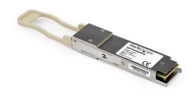
The 40G-QSFP-SR4-ST is a Brocade 40G-QSFP-SR4compatible fiber transceiver module that has been designed, programmed and tested to work with Brocade brand switches and routers. It delivers dependable 40 GbE connectivity over fiber cable, for 40GBase-SR4 compliant networks, with a maximum distance of up to 150 m (492 ft.).
