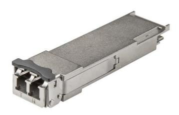
The 40G-QSFP-LR4-ST is a Brocade 40G-QSFP-LR4 compatible fiber transceiver module that has been designed, programmed and tested to work with Brocade brand switches and routers. It delivers dependable 40 GbE connectivity over fiber cable, for 40GBase-LR4 compliant networks, with a maximum distance of up to 10 km (6.2 mi).
