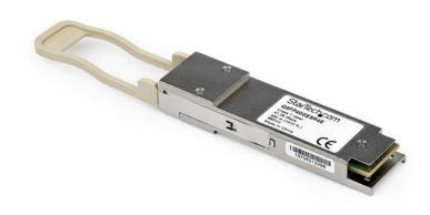
The JG325B-ST is an HP JG325B compatible fiber transceiver module that has been designed, programmed and tested to work with HP brand switches and routers. It delivers dependable 40 GbE connectivity over fiber cable, for 40GBase-SR4 compliant networks, with a maximum distance of up to 150 m (492 ft).
