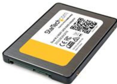
Boost your system performance by enhancing the capacity, speed and security of your data storage. This two-drive M.2 to SATA adapter lets you install two M.2 solid-state drives in a single 2.5" drive bay and configure a powerful RAID array.
