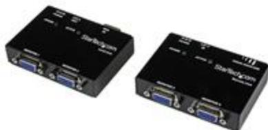
The ST121UTP VGA Video Extender over Cat5 allows you to extend your VGA video signal by up to 150 meters (500 feet) and connect up to 4 displays (2 local and 2 remote) from that single source. The ST121UTP is a bundled kit including both a local transmitter and a remote receiver unit, offering a complete solution for scenarios in which remote monitor displays are required.
