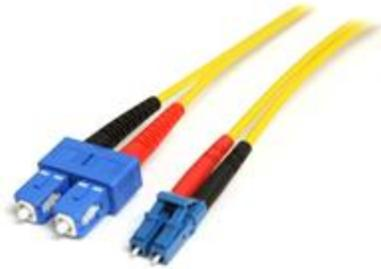
The SMFIBLCSC7 7m LC to SC Single-Mode Duplex Fiber Cable features 9/125 micron fiber for high-speed, high bandwidth data transmissions over Gigabit Ethernet and Fiber Channel networks, with support for duplex single-mode applications.
